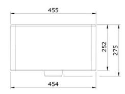
NB: Due to manufacturing processes this sink may have a +/- 5mm tolerance on the measurements.
