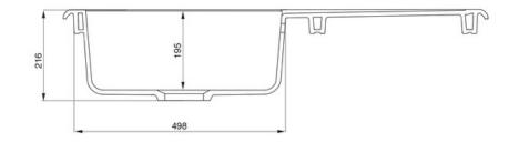
NB: Due to manufacturing processes this sink may have a +/- 3mm tolerance on the measurements.
