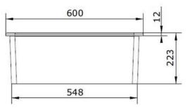
NB: Due to manufacturing processes this sink may have a +/- 3mm tolerance on the measurements.
