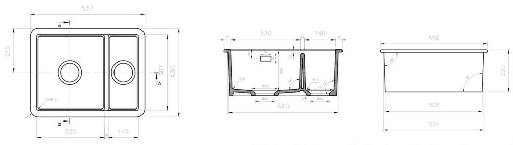
NB: Due to manufacturing processes this sink may have a +/- 4mm tolerance on the measurements.
