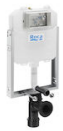
BASIC WC COMPACT - Concealed structure with compact cistern (8 cm) and dual flush (4/2 - 4.5/3 - 6/3 L). 90 ø / 110 ø elbow
