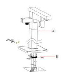
5. Screw the floor anchor to floor and fix it.
