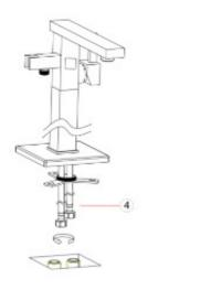
Screw the leg to the Floor anchor(with base plate on).
