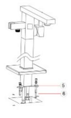
Connect the hose pipe to both ends of Showerhead and the Body.
