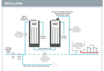
Additional storage tanks must be the same capacity as the main TankBoost unit. The tanks must be located next to each other and on the same level. The total volume of stored water must not be more than will be used in a single day. The supplied tank connector kit should be used to link the tanks.
