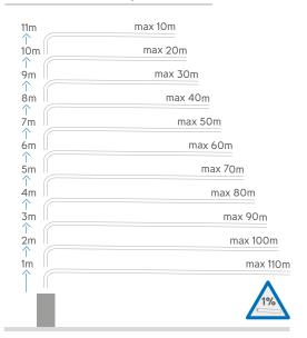
Max pumping height 14m at 0 flow rate
