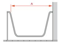
NB Screen must be set 10mm in from the bath edge in order for rubber seal to be water tight.
