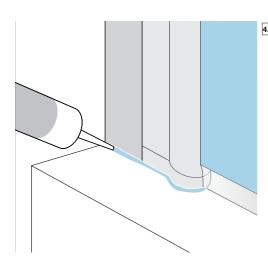
[4.1] Using a silicone based sealer (always check product instructions to check if suitable), seal along the outside edge of the vertical fixing rail and the wall, as well as between the outside bottom of the screen frame and the bath.
