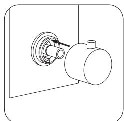
Fit temperature control handle to thermostat, ensuring the stop pin inside the handle, is located against the top of the stop ring.
