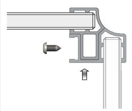
Corner Profiles to be pushed & held together firmly during fixing. Ensure both panels are plumb & top edges are aligned. Carefully drill (dia 3mm) & screw corner profiles together.
