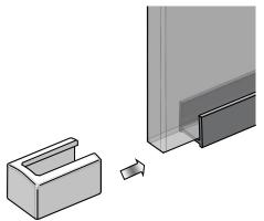
'Fit corner piece to bottom corner of 'open' glass edges. Clear silicone may be used to retain ~ wipe off excess. If a foot is to be used, see Foot Kit instructions (Fig C)
