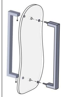
Assemble handle to glass as shown (handle with pins to outside).
