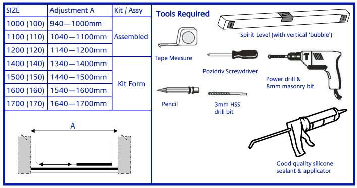
Lakes Coastline Sliding Door is fully reversible, so suitable for fitting with door to left or right hand side of enclosure. Ensure tray is correctly levelled & that all tray/wall joints are sealed & cured over entire length of tray sides (See — — — — Fig A) prior to fitting enclosure.
