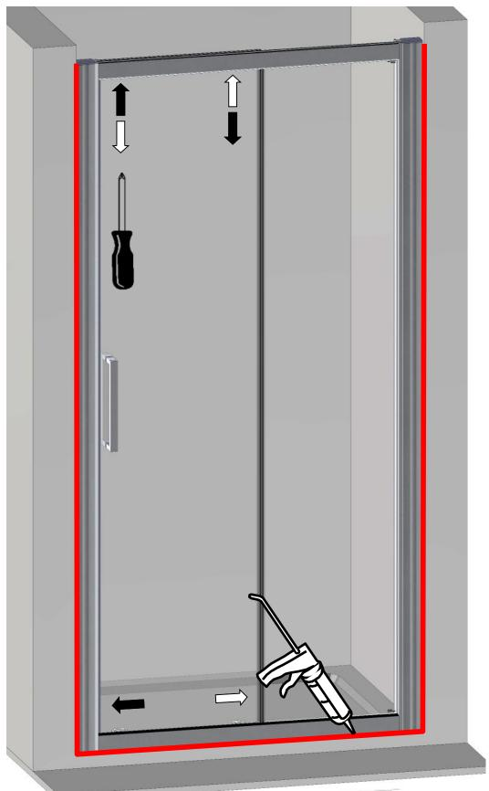
From underside of top wheels, adjust door height until bottom wheels are engaged in horizontal profile (no wobble). Then adjust door angle plumb with vertical frame profiles (check door edge contact with bump stop).
