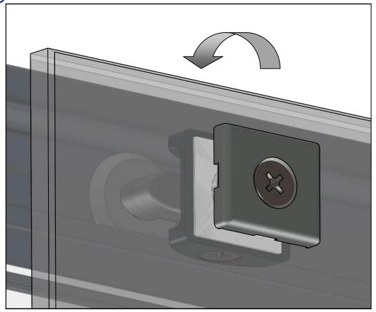
Carefully lift door into enclosure & engage top wheels into wheel groove. (If necessary loosen, but do not remove centre screw to permit engagement). Immediately after all wheels are correctly engaged, fully tighten centre screw to retain door. Fit internal wheel covers \*\*.
