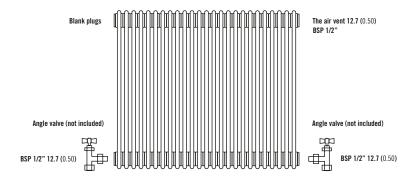
Note: Factory fitted bushes are welded in place and not removable If installing TBOE (Top Bottom Opposite End) please note that the radiator MUST be inverted.
