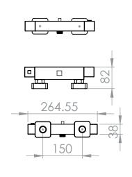
Diagrams not to scale All dimensins in mm tolerance of +5mm
