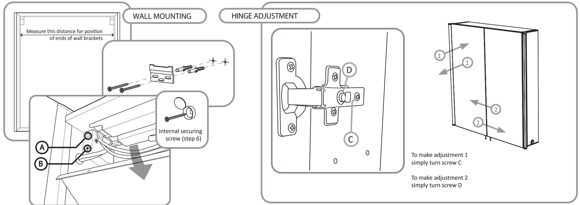
**1)** Remove the packaging taking special care with the doors and separate shelves. Open the cabinet doors and ensuring you haven't connected the power remove the screws on the front edge and lower the cover. Take care not to lose the screws.
