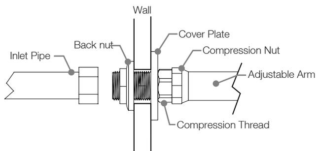
1. Secure arm in place using the back nut provided (See diagram above)
