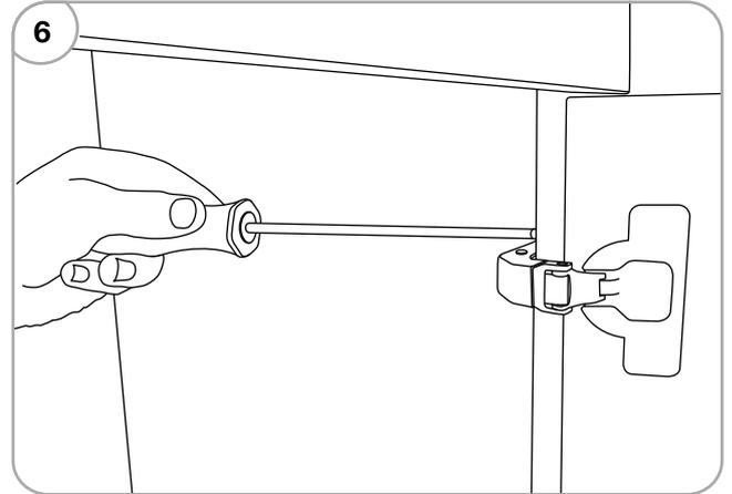
If the delivered configuration isn't suitable, remove door and hinge plates from unit using a suitable tool.
