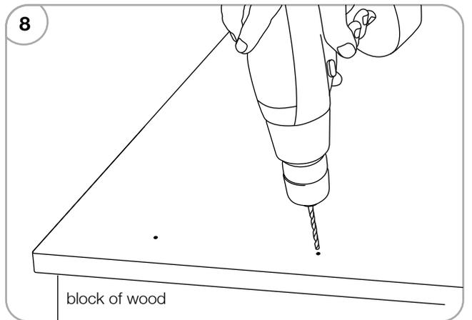
Once the handing has been chosen, remove the door using the quick release hinges. Place door on to a clean and smooth scrap piece of wood and carefully drill out the selected holes for the handle bolts.
