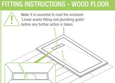
Take care to avoid chipping on bottom edges/corners when moving the tray into position.
