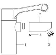
Periodically the spout and nozzle should be removed, cleaned and disinfected to remove any build up of debris, deposits or bio film which may affect the performance of the tap.
