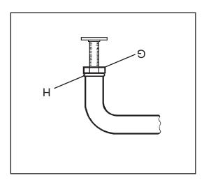
against bushes (H). (5) stun nogsxad gninathgit lock feet in position by lightly from floor to top of bath) and and height (normally 540mm 4. Adjust feet for correct level
