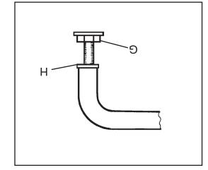
cradles. bushed ends (H) of the adjustable feet into the adjustable feet. Screw the 3. Screw nuts (G) onto the
