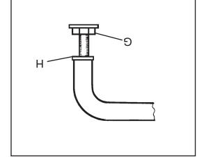
3. Screw nuts (G) onto the adjustable feet. Screw the adjustable feet into the bushed ends (H) of the cradles.
