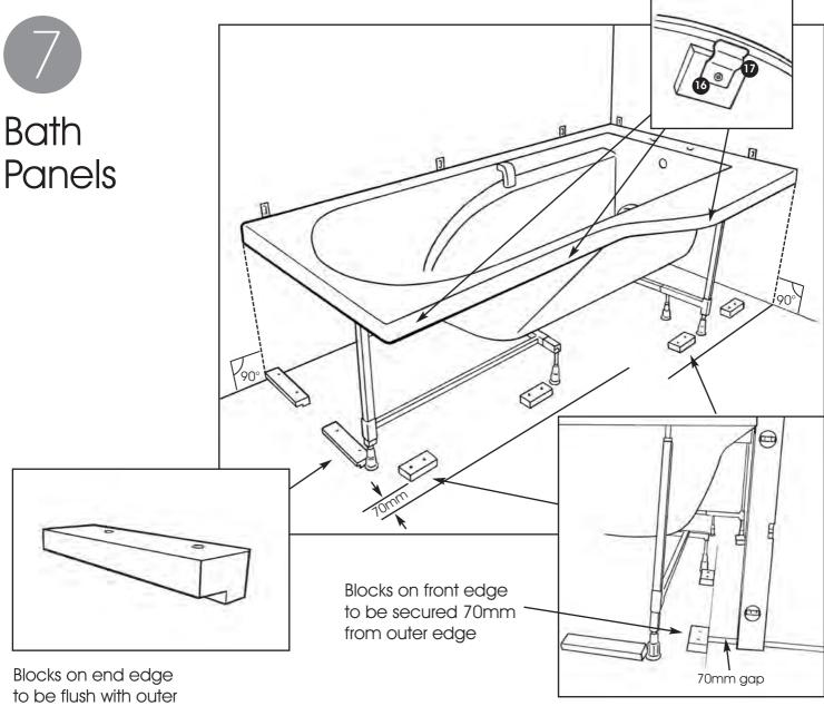
to be flush with outer edge of the bath and need a recess for the bottom return edge of the panel
