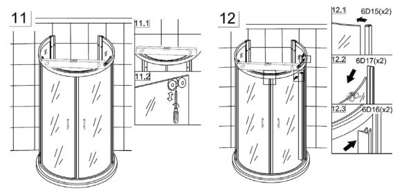
11. Put spirit level on top of sliding panels. Adjust the rollers with driver to make sure sliding door vertical for better sliding effect.
