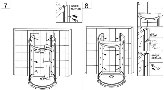
7. Inside of cabin, fasten wall profile on the wall with screw 6D6 and screw cap 6D10.
