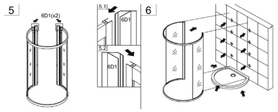
5. Put wall profile 6D1 on the 2 sides of frame.
