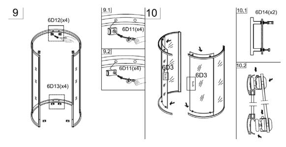
9. Mount stopper 6D12 on top rail profile and 6D13 on bottom rail profile with screw 6D11.
