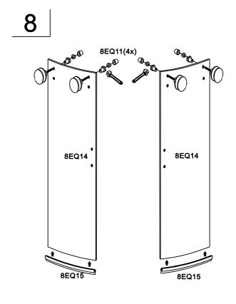
$8.\ Assemble\ rollers\ 8EQ11$  on sliding panel 8EQ14. Attach bottom seal 8EQ15 on the bottom of glass.
