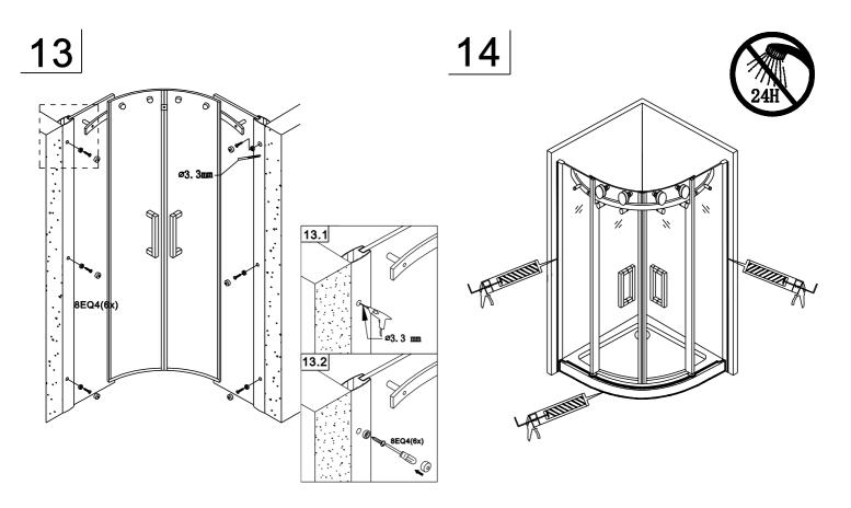
13. Drill the holes (6mm) on vertical profile into wall profile 8EQ3 and door profile. Use rubber washers and screws 8EQ4 to fix them in place. Press the screw caps over screws.
