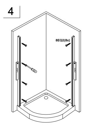
4. Fix the wall profiles 8EQ3 with the St4x30 screws 8EQ2 to the wall.
