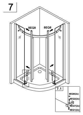
7.Attach the vertical sealer 8EQ8 on the fixing panel 8EQ5. Put the bottom bracket 8EQ7 on the fixing glass panel and mark the hole for the bracket. Drill the holes (6mm) according to the marks and insert the wall plugs 8EQ1 into the holes. Fix the bracket 8EQ7 with the St4x30 screws 8EQ2 to the tray. Put the cover 8EQ6 on screw.
