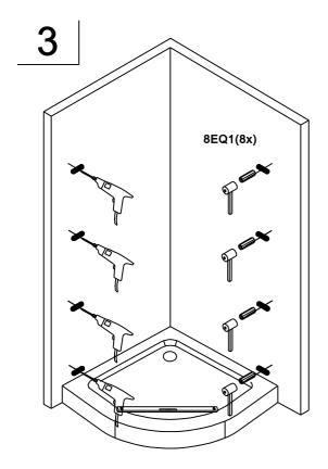
3. Drill the holes ( $\emptyset$ 6mm) according to the marks and insert the wall plugs 8EQ1 into the holes.
