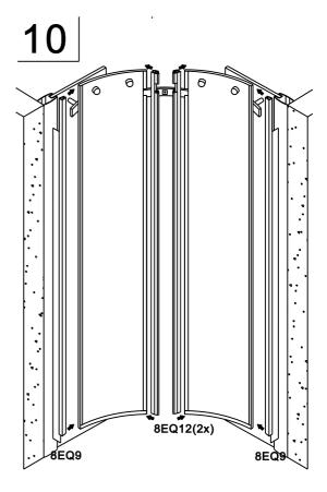
10. Attach magnetic strip 8EQ12 to sliding panel 8EQ14. Attached vertical sealer 8EQ9 to the other side of sliding panel.
