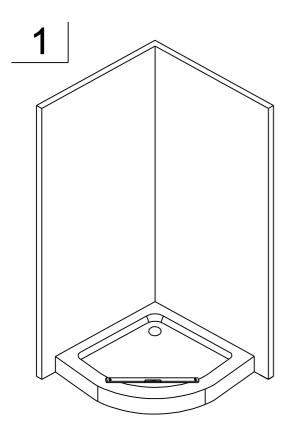
1. If the quadrant is placed onto a tray, first take a spirit level to check whether the tray is placed horizontal. In case the quadrant is installed directly onto the floor, please proceed with step 2.
