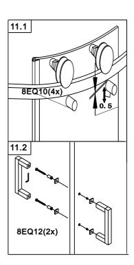
11. Assemble the fixing part 8EQ10 on sliding panel below rail profile. 8EQ10 is eccentric. Adjust the distance between rail profile and 8EQ10 to be 0.5mm.
