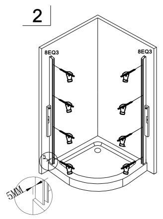
2.Put the wall profiles 8EQ3 against the wall, ensuring the distance between the profile and the wall is correct. Please make sure profile to be 5mm away from outside edge. Adjust the profile to make sure it is vertical by using a spirit level. Mark the holes on the wall.
