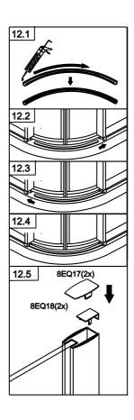
12. Put silicon glue on the back of bottom aluminum strip 8EQ16. Put it on the tray edge between brackets 8EQ7. Put the profile cover 8EQ18 on the vertical profile and put profile cover 8EQ17 on the wall profile.
