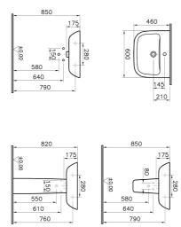
All drawings contain the necessary measurements which are subject to standard tolerances. For exact measurements, in particular for customized installation scenarios, it can only be taken from the finished ceramic product.
