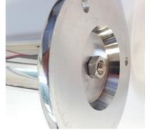
Now tighten the M6 Nut (finger tighten the nut then ¼ turn with the spanner.)
