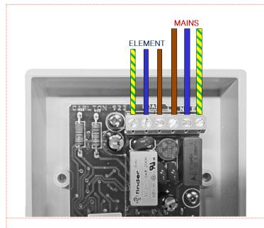
Clamp the element cable to the bottom of the wall controller
