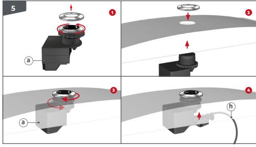
INSTALLING THE SENSOR ③: • Unscrew the chrome fascia by rotating anti-clockwise. • Position the sensor through the cistern lid. • Replace the chrome fascia by rotating clockwise 1/4 turn. Secure in place with the nut. • Clip the cable mechanism to the sensor.
