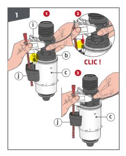
ATTACHING THE FLOAT: Position the float 1 as shown in the diagram and the fork 1 on the narrow side of the overflow 6.
