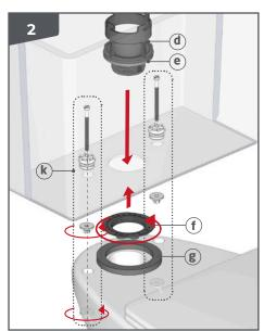
ATTACHING THE BASE: Place e and e at the bottom of the tank. Tighten the nut f. Center g on the basin. Secure the tank with the screws e.
