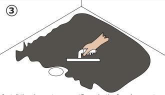
Install the shower tray on a 15mm depth of weak cement mix (sand/cement ratio 5:1). Tile adhesive can be used as an alternate to sand or cement.
