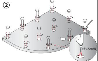
Using the appropriate foot as a guide mark with a pencil the fixing hole positions, and then using a 3.5 diameter bit drill to a maximum depth of 5mm. DO NOT OVER DRILL PAST THE 5MM DEPTH.
