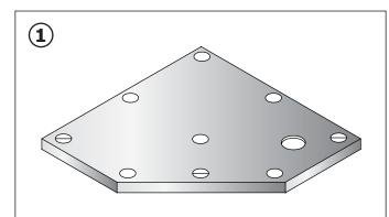
Turn the tray over and use the cardboard packaging as a protective mat. Note the circles that have been marked to indicate feet position. The symbol  $\bigcirc$  indicates where you should fix the feet with the panel fixing rod.
