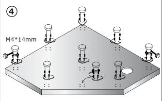
Screw the feet in position with the screws provided. Ensure that the feet that have panel fixing rod attached, are placed around the bended edge where the panel will meet.
