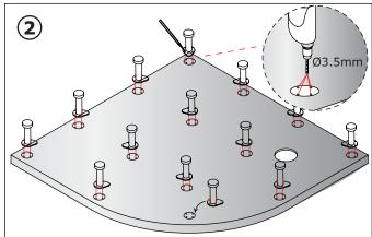
Using the foot as a guide mark with a pencil the fixing hole positions, and then using a 3.5 diameter bit drill to a maximum depth of 5mm. DO NOT OVER DRILL PAST THE 5MM DEPTH.
