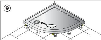
When shower tray is set remove the remainder of the protective plastic film and connect the waste pipe and check for leakage and water drainage.
