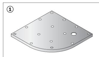
Turn the tray over and use the cardboard packaging as a protective mat. Note the circles that have been marked to indicate feet position. The symbol igopoonup indicates where you should fix the feet with the panel fixing rod.
