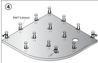
Screw the feet in position with the screws provided. Ensure that the feet that have panel fixing rod attached, are placed around the curved edge where the panel will meet.
