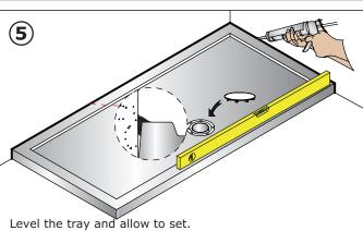
When shower tray is set remove the remainder of the protective plastic film and connect the waste pipe and check for leakage.
