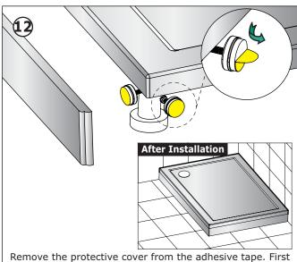
Remove the protective cover from the adhesive tape. First fix the rebated panel pushing it firmly on to the adhesive pads. Then fix the remaining panel in the same manner.
