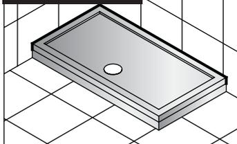
Remove the protective cover from the adhesive tape. First fix the rebated panel pushing it firmly on to the adhesive pads. Then fix the remaining panel in the same manner.
