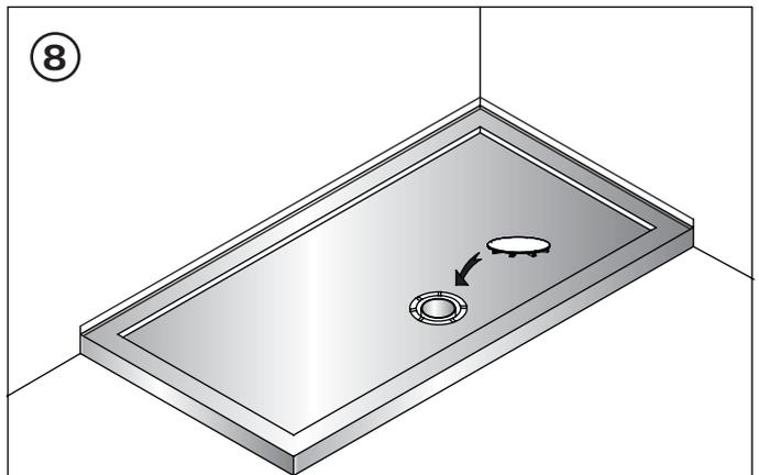
When shower tray is set remove the remainder of the protective plastic film and connect the waste pipe and check for leakage and water drainage.
