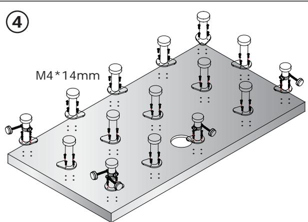
Screw the feet in position with the screws provided. Ensure that the foot that has two panel fixing rods attached, is placed in the corner where the panels will meet.
