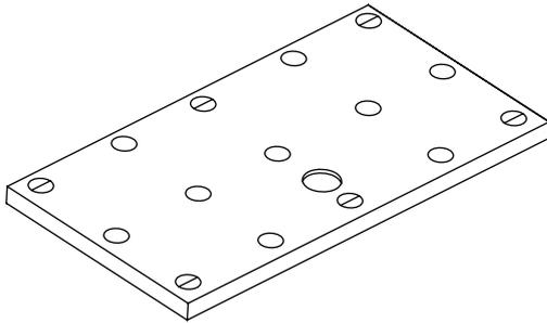
Turn the tray over and use the cardboard packaging as a protective mat. Note the circles that have been marked to indicate feet position. The symbol ⊕ indicates where you should fix the feet with the panel fixing rod, but for the symbol ⊖ you will only use four of these positions and the other two would be supplemented with the feet without the panel fixing rod.
