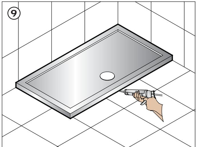
Tile and seal joints with an anti fungal silicone sealant and allow to set.
