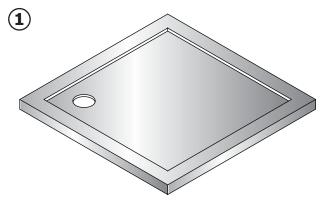
Remove protective plastic film from the areas near the waste and those sides of the tray which will be against a wall.
