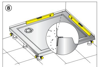
Ensure the 'easyseal' water sealing strip is flat to the wall. Place the tray into position and level both ways using the legs. After the tray has been levelled adjust all the inner feet to stabilise the tray. When level fix these legs to the floor with silicon sealant or 'no more nails' type adhesive.
