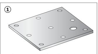
Turn the tray over and use the cardboard packaging as a protective mat. Note the circles that have been marked to indicate feet position. The symbol  $\bigoplus$  indicates where you should fix the feet with the panel fixing rod, but for the symbol  $\bigoplus$  you will only use three of these positions and the fourth would be supplemented with a foot without the panel fixing rod.
