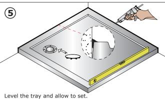
When shower tray is set remove the remainder of the protective plastic film and connect the waste pipe and check for leakage.
