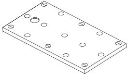
Turn the tray over and use the cardboard packaging as a protective mat. Note the circles that have been marked to indicate feet position. The symbol  $\bigcirc$  indicates where you should fix the feet with the panel fixing rod, but for the symbol  $\bigcirc$  you will only use four of these positions and the other two would be supplemented with the feet without the panel fixing rod.
