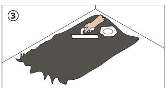
Install the shower tray on a 15mm depth of weak cement mix (sand/cement ratio 5:1). Tile adhesive can be used as an alternate to sand or cement.
