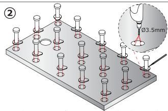
Using the appropriate foot as a guide mark with a pencil the fixing hole positions, and then using a 3.5 diameter bit drill to a maximum depth of 5mm. DO NOT OVER DRILL PAST THE 5MM DEPTH.
