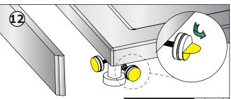
Remove the protective cover from the adhesive tape. First fix the rebated panel pushing it firmly on to the adhesive pads. Then fix the remaining panel in the same manner.
