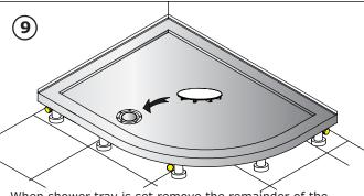
When shower tray is set remove the remainder of the protective plastic film and connect the waste pipe and check for leakage and water drainage.
