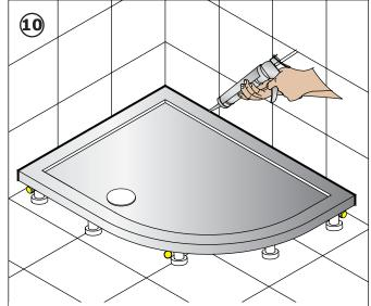
Tile the wall and seal joints with an anti fungal silicone sealant and allow to set.
