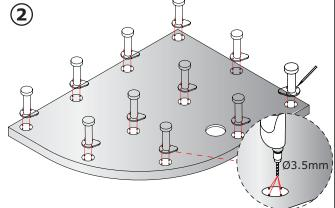
Using the appropriate foot as a guide mark with a pencil the fixing hole positions, and then using a 3.5 diameter bit drill to a maximum depth of 5mm. DO NOT OVER DRILL PAST THE 5MM DEPTH.
